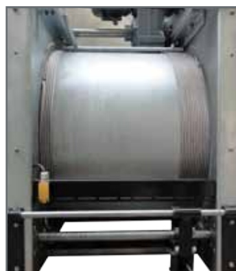
Drum (Ø 800 mm) with single-layer coiling on the left and on the right side
